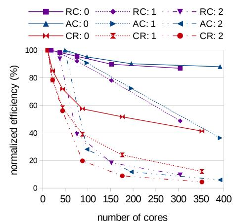
RC=Replication/resampling AC=Alternate recombination CR=Checkpoint/Restart
